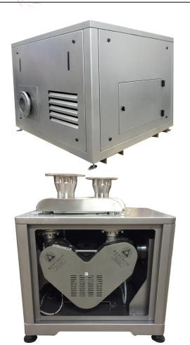
**REPUBLIC'S ENCLOSURES** reduce the noise transmitted by the blower while protecting the blower from the elements. Available in stainless steel or aluminum, the enclosure includes a ventilation fan to protect the blower from overheating. All gauges are visible externally and maintenance items are easily accessible by hinged doors.
